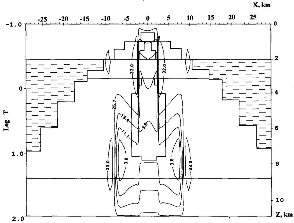
Figure 2. Pseudosection of  $\phi_{xy} (\times 10^{-1})$  for volcano model shown in Fig. 1.
