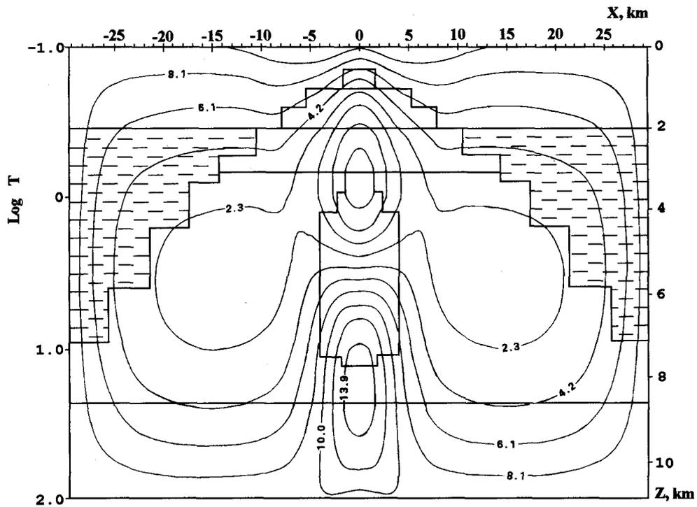
Figure 4. Pseudosection of  $\text{Re } E_y$  ( $\times 10^1$ ) for volcano model shown in Fig. 1. Result is based on an incident electrical field, parallel to y-axis.
