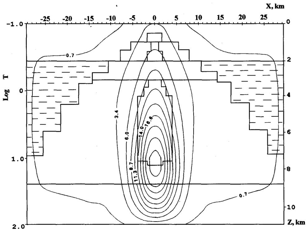
Figure 5. Pseudosection of  $\text{Im } E_y$  ( $\times 10^1$ ) for volcano model shown in Fig. 1. Result is based on an incident electrical field, parallel to y-axis.
