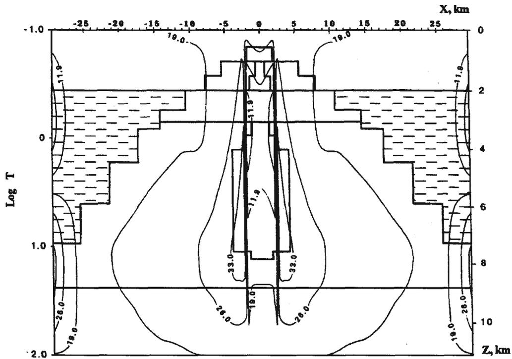
Figure 3. Pseudosection of  $\phi_{det} (\times 10^{-1})$  for volcano model shown in Fig. 1.
